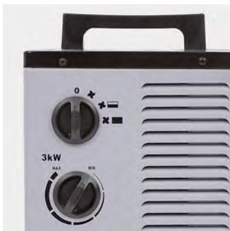
Due to their thermally insulated carrying handle the fan heaters of the TDS-P series can easily be transported to the installation site, started up in thermostat-controlled automatic mode, and fine-adjusted by means of two selectable heating levels, while the cold air level additionally allows for ventilation without heating.
