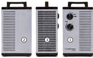
Two air inlets at the front (1) and rear (2) of the heating device supply the powerful radial fan with a high volume of intake air that is then released to the room as warm air current blown through the lateral discharge grille (3).
