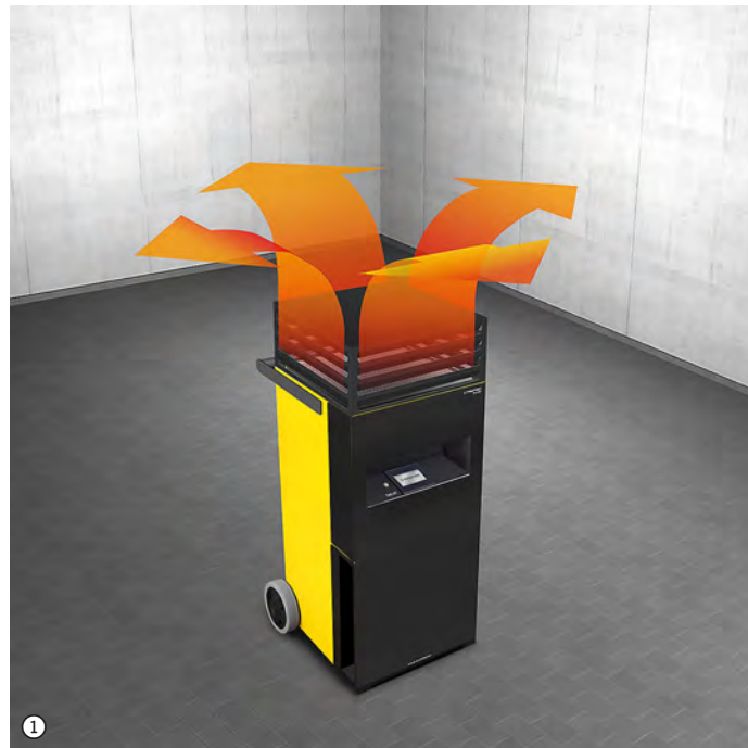
As standard, the DualDecon blowing-out tower ① provides for draught-free warm air throughout the room with a working radius of 360°. The attachment hood for hose connection is optionally available and can be used for central room heating, e.g. of workshops or warehouses, by connecting an optional fabric air distributor ② or the TAC XT to existing ventilation systems ③.
